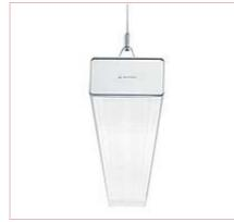
Indirect/direct luminaire with MPO micropyramidal optic, with digitally dimmable electronic ballast, DALI controllable luminaire for T16 lamp, 1/54 W. Direct light component guided via singlepiece MPO-plus micro-pyramidal optic; ...
