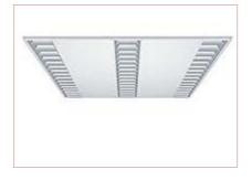
Recessed DALI controllable luminaire for 3/14 W lamps, with reflector optic made of mat silver anodised pure aluminium, with digitally dimmable electronic ballast, ...
