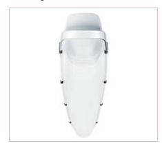
Moisture-proof diffuser luminaire 1/49W T16, with electronic ballast; fibreglass reinforced polyester housing, halogen-free, light grey; PC (polycarbonate) diffuser made as a single injection-moulded piece patterned with internal prisms; fitted to ceiling, wall or trunking using V2A standard spring clips; ...
